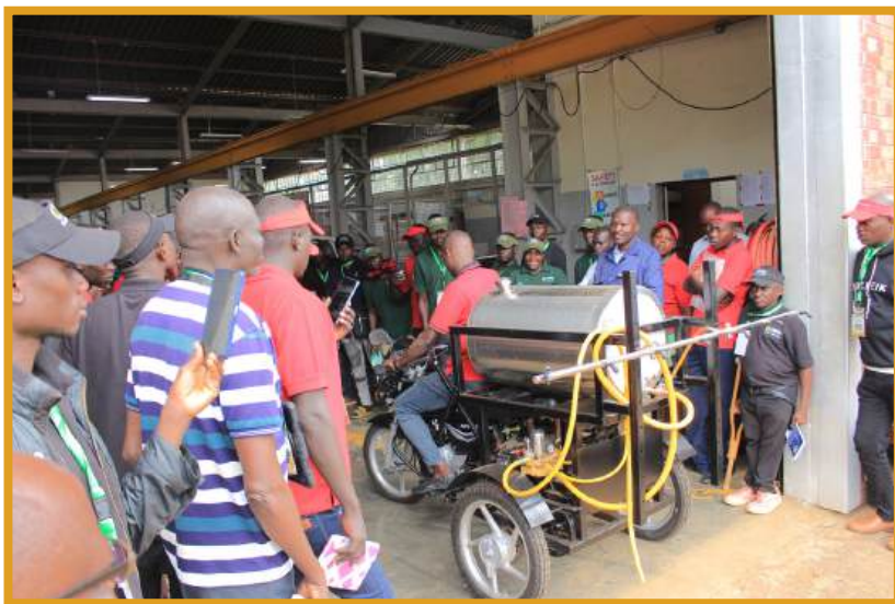
A student demonstrating his innovation of a mobile irrigation / straying system made out of a modified motor cycle and other simple local materials.
